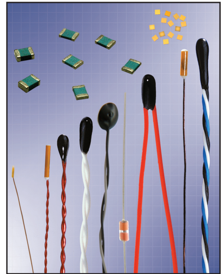
Figure 1. NTC thermistors are manufactured in a variety of sizes and configurations. The chips at the top of the photo can be used as surface mount devices or attached to different types of insulated or uninsulated wire leads. The thermistor element is usually coated with a phenolic or epoxy material that provides protection from environmental conditions. For applications requiring sensing tip dimensions with part-to-part uniformity and/or smaller size, the devices can be encapsulated in PVC cups or polyimide tubes.
